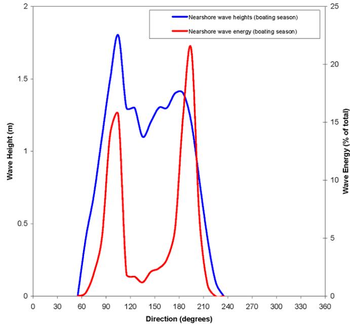
Figure 3.9 Wave Height Decay
