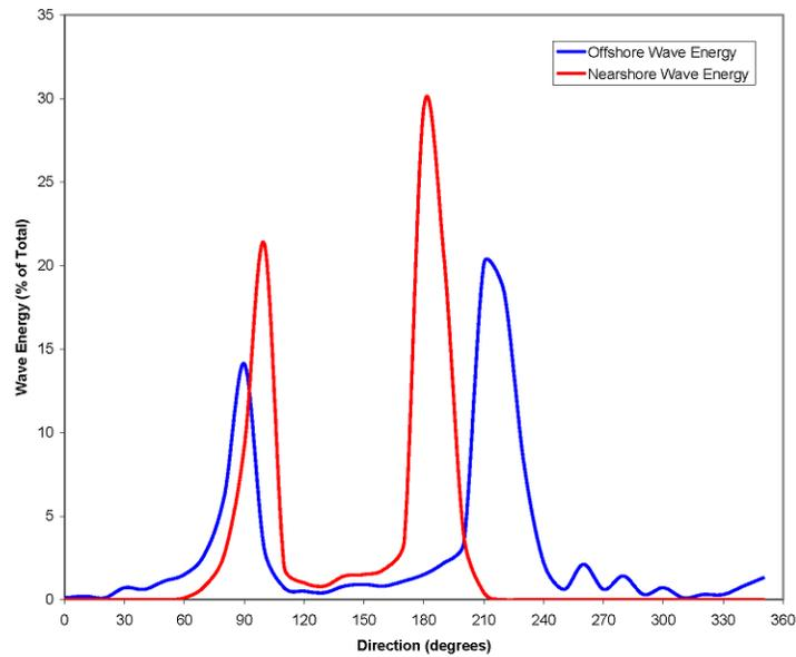
Figure 3.8 Directional Distribution of Nearshore Wave Height and Wave Energy (Boating Season)
