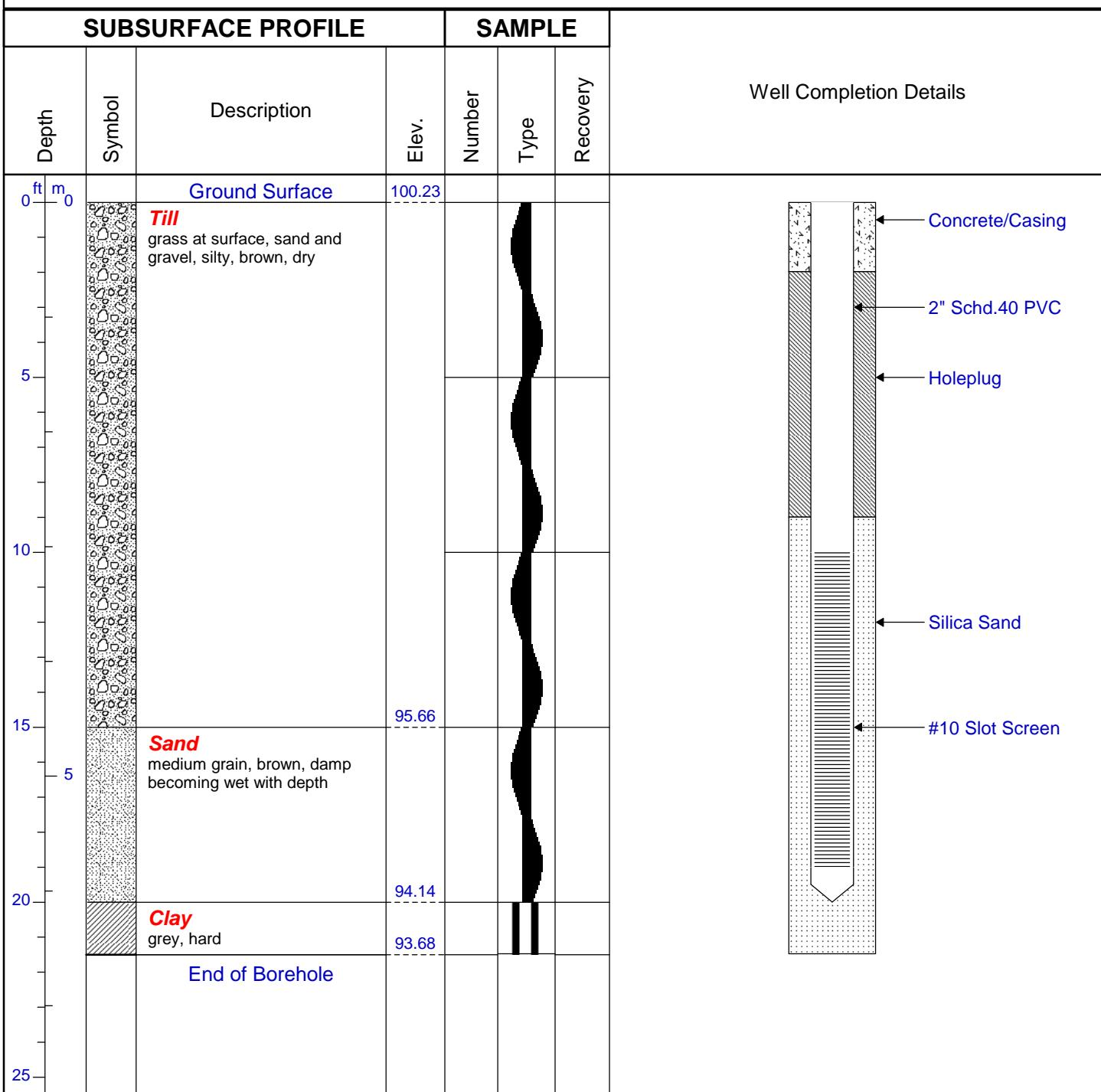
Drill Method: Hollow Stem Auger
