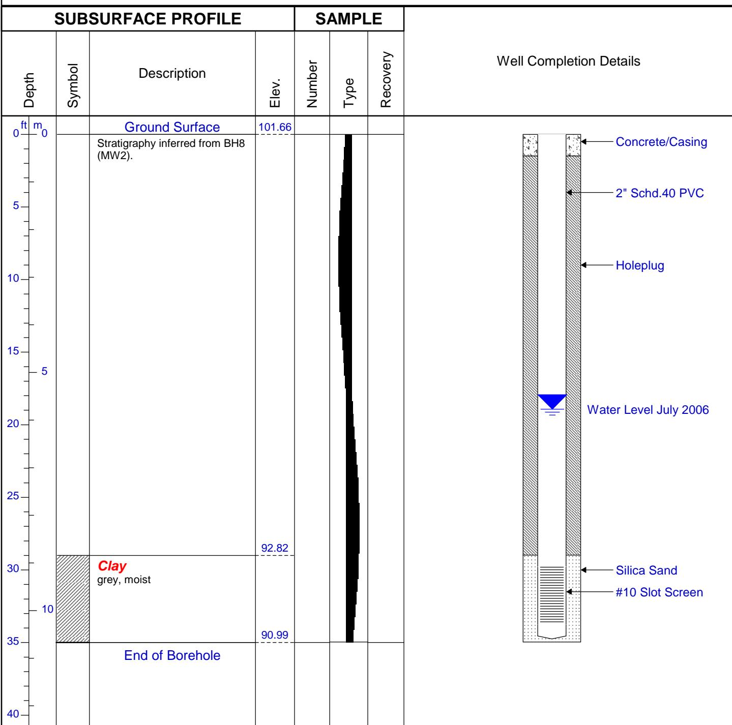
Drill Method: Hollow Stem Auger
