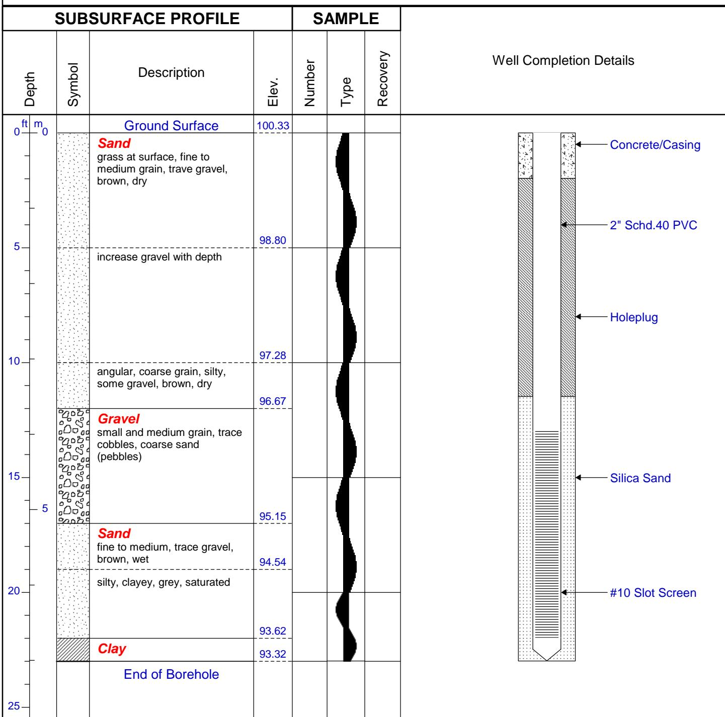
Drill Method: Hollow Stem Auger
