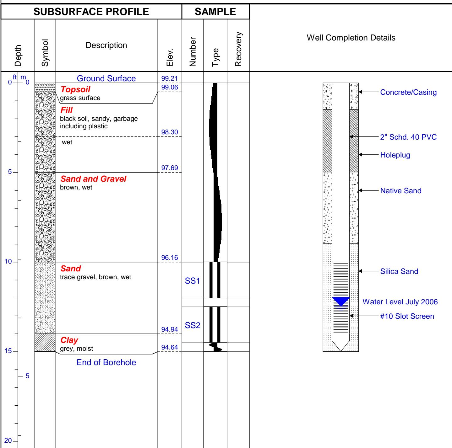
Drill Method: Hollow Stem Auger
