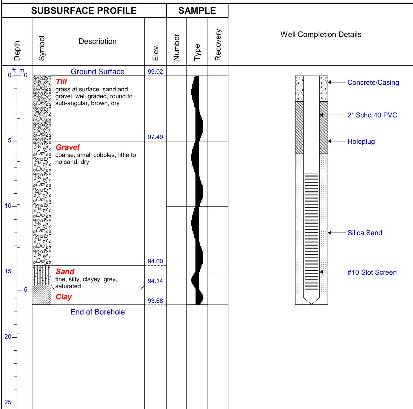
Drill Method: Hollow Stem Auger
