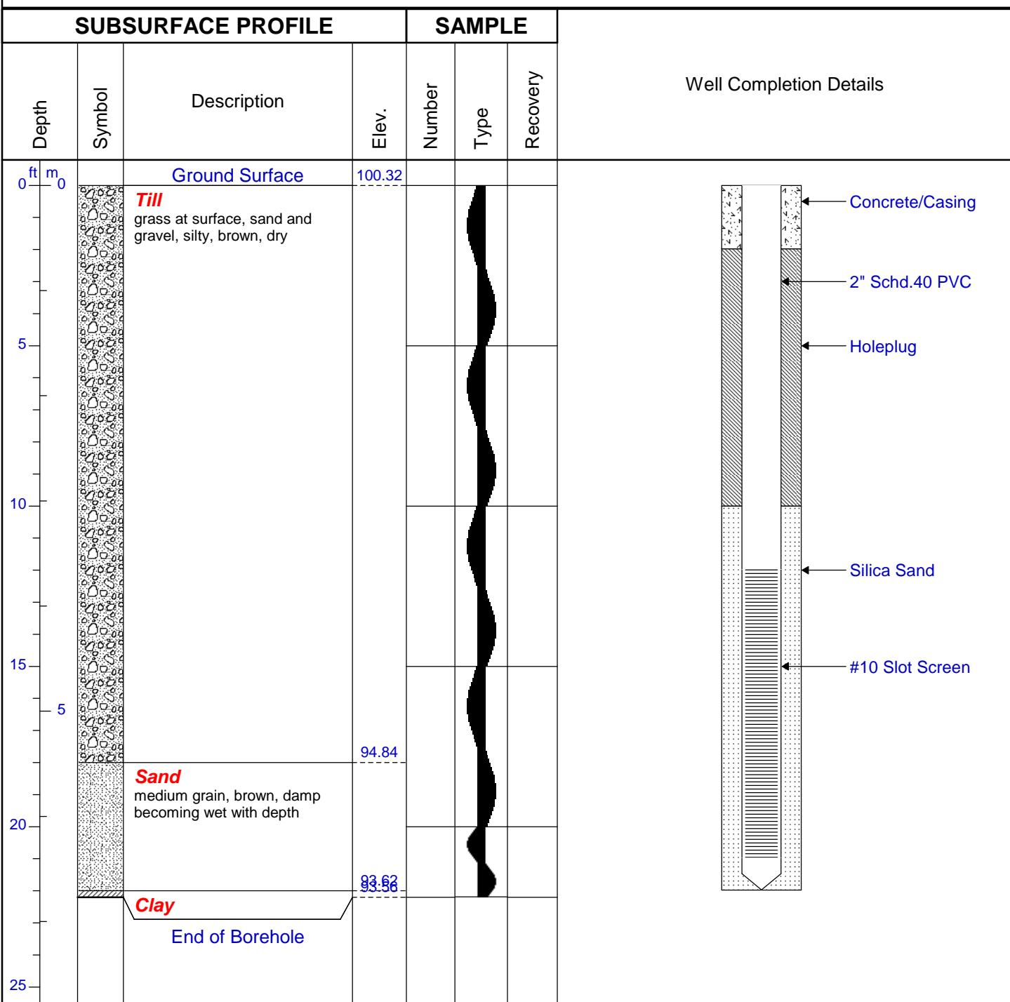
Drill Method: Hollow Stem Auger
