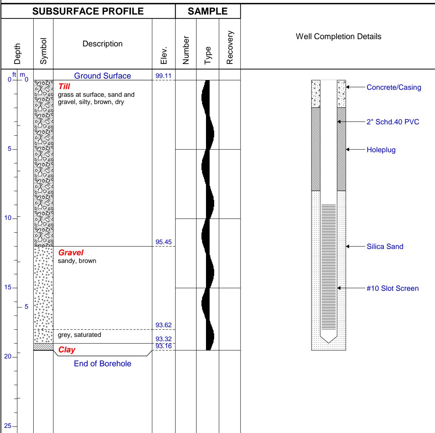
Drill Method: Hollow Stem Auger
