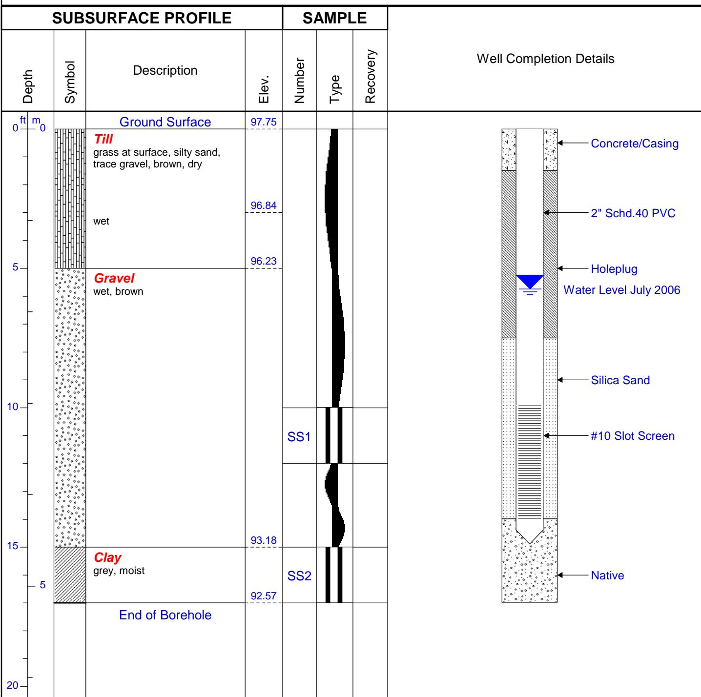
Drill Method: Hollow Stem Auger
