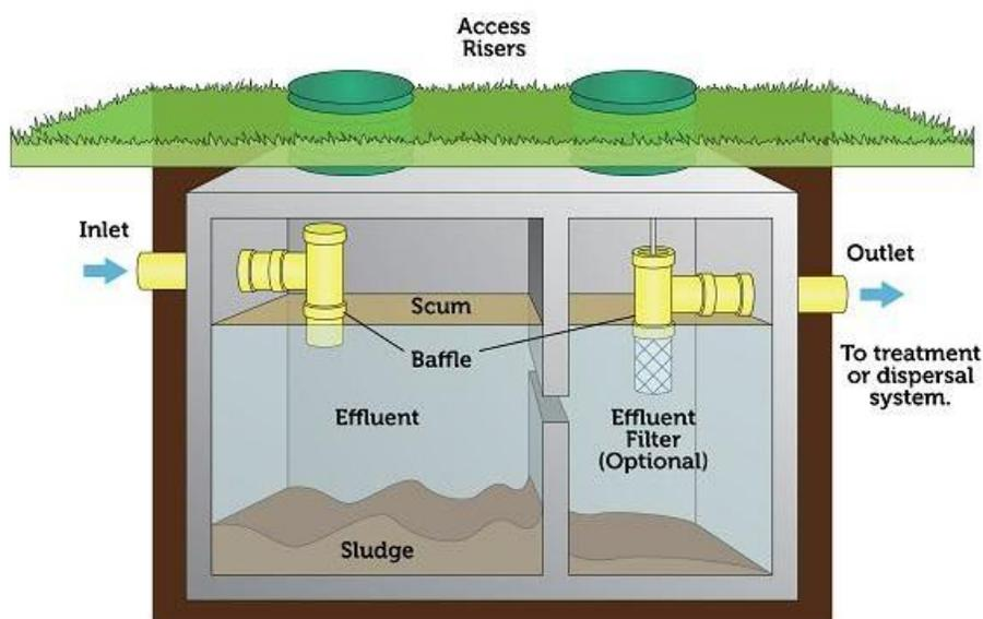
Figure 2.2 – Typical Two-Compartment Septic Tank (obtained from US EPA)
